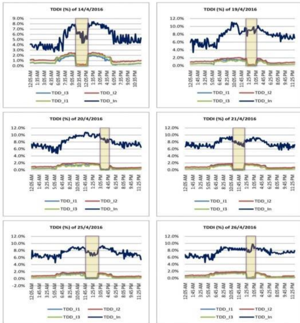
Fig. 5.8 TDD (%) of phase and neutral currents for the days in which the system was down during monitoring period “1”
